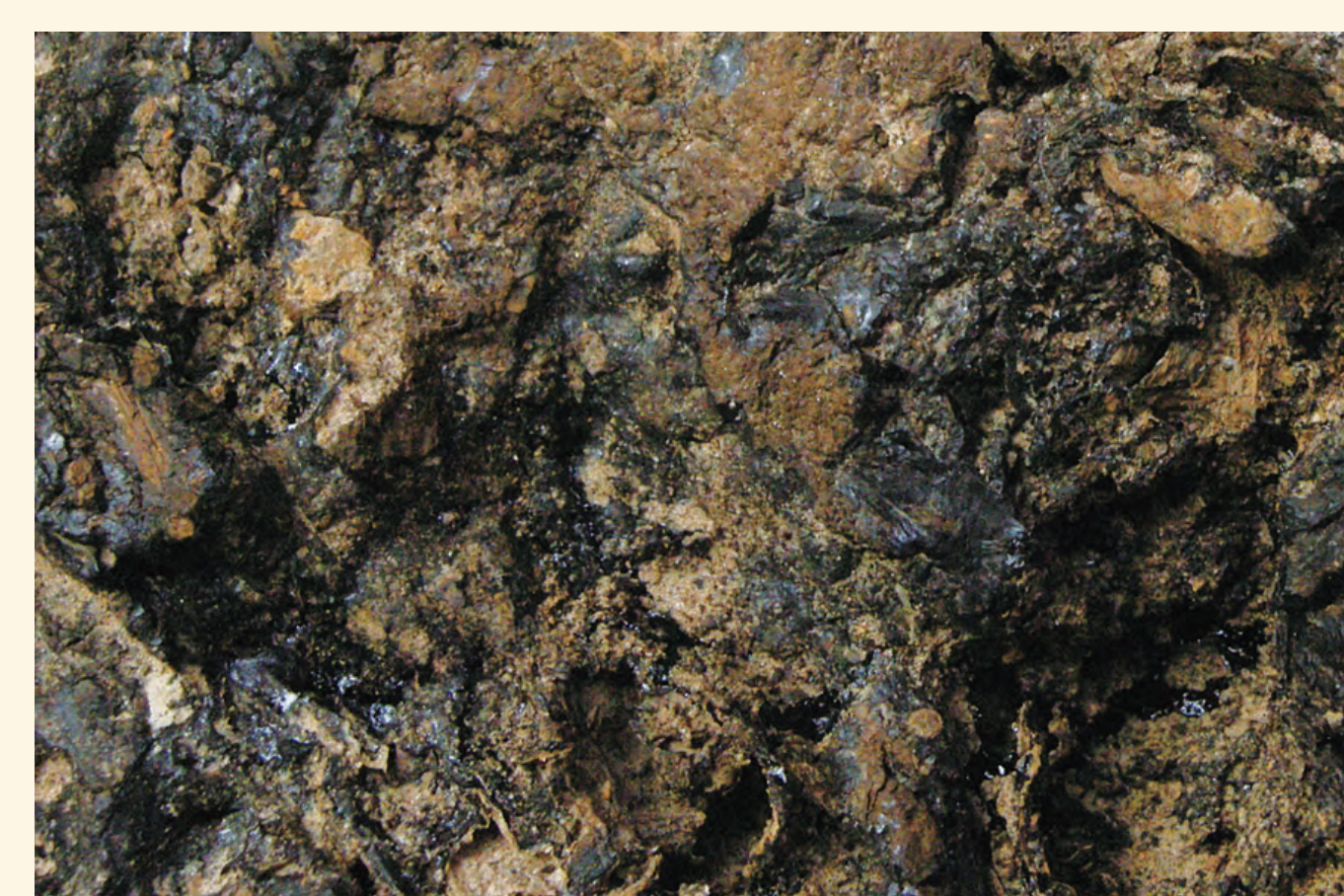
Asphalt containing a lot of impurities (magnified view on the right)
